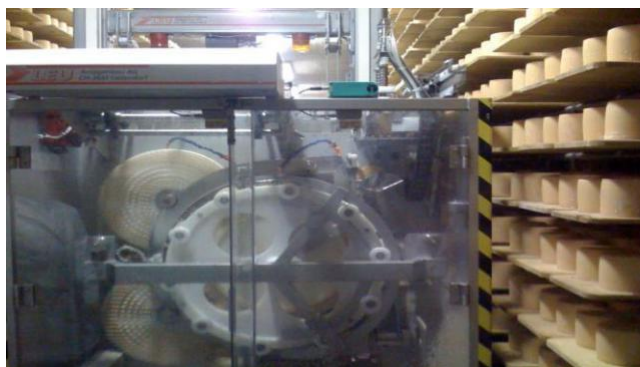
PhageGuard Listex is applied at the point of smearing/washing which potentially is a vulnerable point in the process.
